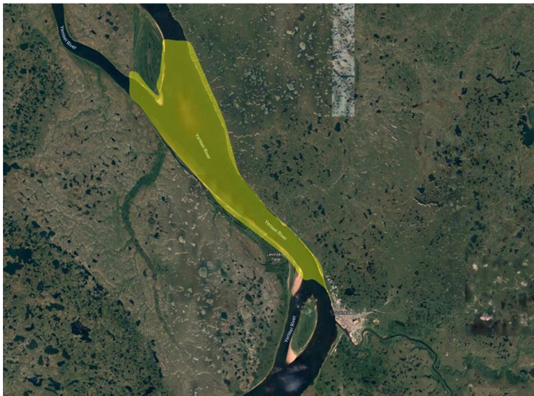
Figure 1. Simulated area of bottling of oil products 4 hours after entering the reservoir (scale 1: 25000)
