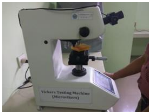
Figure 03. Microvikers FM 800 for hardness test
