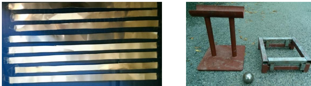
Figure 01. (a) Shape of continuous waste cans fiber and (b) drop weight test jig
