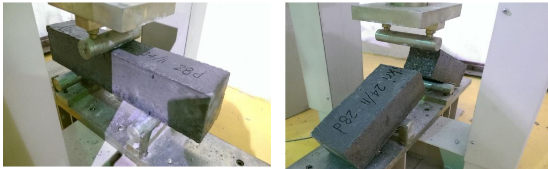
Figure 02. Beam under flexural load (a), and beam failure (b)
