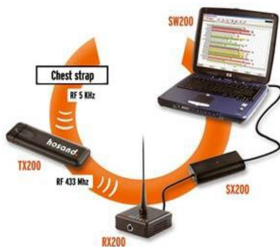
Fig. 1. Component parts of HOSAND telemetry system
