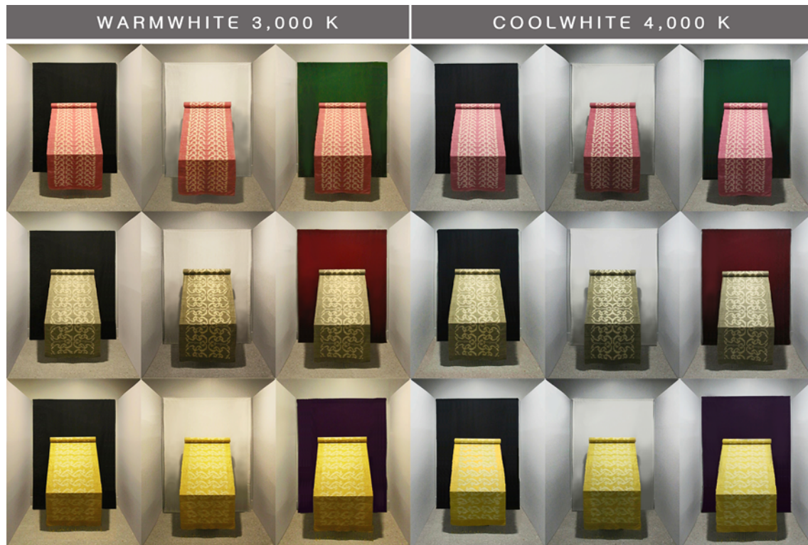
Figure 01. Six conditions of each sample fabric in the experiment
