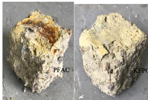
Figure 04. PFAC and KFPC samples after 365 days acid immersion
